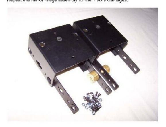
Prepare the Couplings by disassembling the rubber from the metal ends and epoxy back together. Also check the fit of the Coupling to the Threaded Drive Screw. File the reduced diameter of the Drive Screw to fit into the Coupling. Assemble the Motor Coupling to the shaft of a Stepper Motor. Tighten the setscrew to the flat on the Stepper Motor Shaft.
