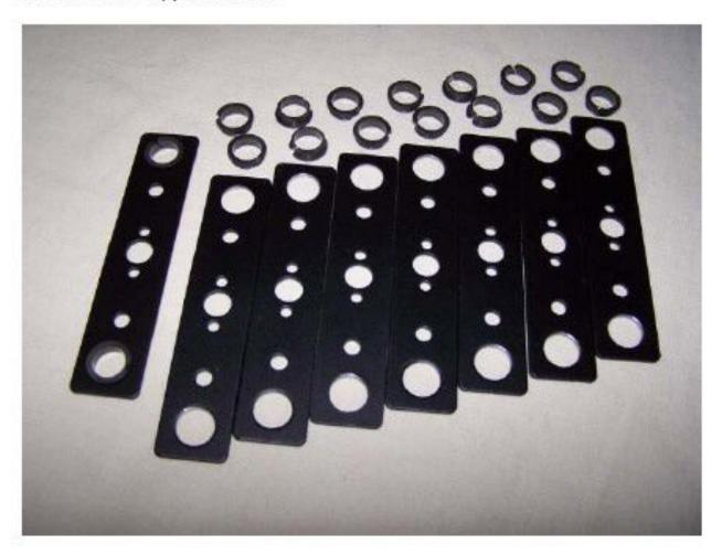
Install the Lead Nut onto a Support Plate with 8-32 screws on the opposite side of Teflon Bushing large flange. Assemble 4 Support Plates.
