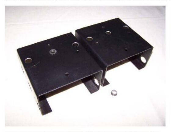
Install 1 small Teflon Bushing into the face of the End Mounting Bracket.
