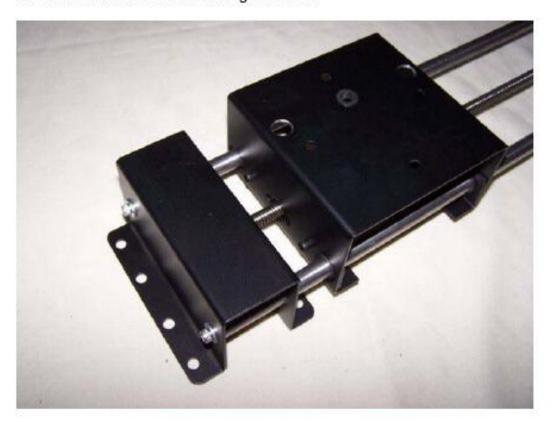
Set an X Axis assembly on the flat surface of a table. Tighten ONLY the Guide Rod Screws. The Support Plate Screws will be tightened AFTER you have run the machine to its extreme several times. Adjust 2 X Axis Assemblies.
