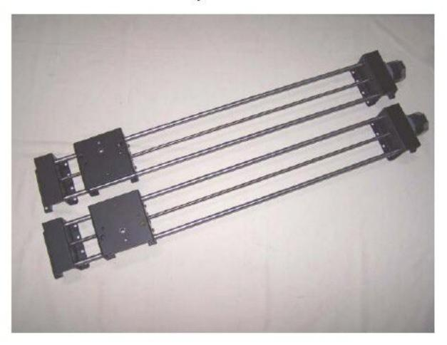
Position an X Axis Assembly and a Y Axis Assembly on their sides. Slide the Guide Rods and Drive Screw of the Y Axis Assembly into the holes of the X Axis Carriage. Attach with 10-32 screws and washers and tighten. Tighten screws of 2 X Axis Assemblies.
