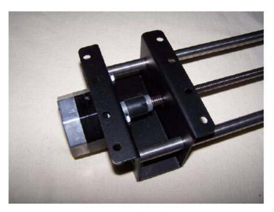
Slide an End Mounting Bracket onto the end of the Guide Rods of an X Axis Assembly. Attach with 10-32 screws and washers but do not tighten the screws. Assemble 2 X Axis End Mounting Brackets.
