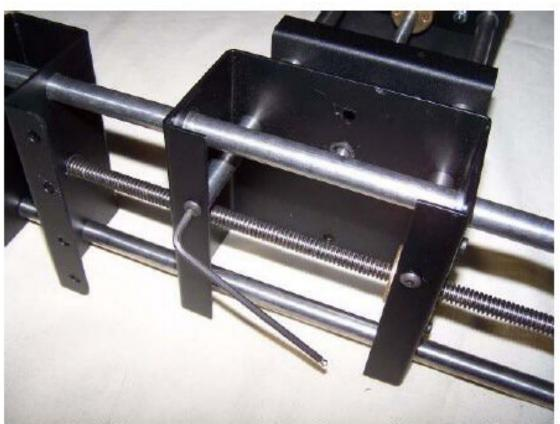
Position the XY Towers at each end of a table about 5 feet apart with the face of the Y Carriage facing each other. Secure with customer supplied bolts and nuts. (An alternative way is to mount each XY Tower to a board with bolts and nuts. The towers then can be positioned apart as desired and secured with clamps – and repositioned easily as a setup dictates.)
