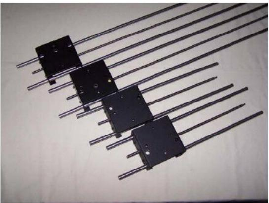
Slide a Motor Mount Bracket onto the Guide Rods of an X Axis Assembly. (End with the reduced diameter Drive Screw.) Attach with 10-32 screws and washers but do not tighten the screws. Tighten the Motor Coupling screw securely to the Drive Screw reduced diameter. The holes/Guide Rods are a tight fit – use a brass hammer. Assemble 2 X Axis Motor Mount Brackets, Assemble 2 Y Axis Motor Mount Brackets.
