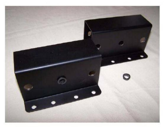
Install 1 Support Plate / Lead Nut and 1 Support Plate / no Lead Nut to the inside of an X Axis Carriage using 8-32 screws. Leave the screws loose for later alignment. Assemble the other X Axis Carriage in such a manner so that you make a mirror image of the first X Axis Carriage.
